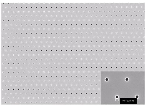
Nanohole array printed on the Phabler 100 DUV tool (hole period = 600nm)
